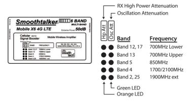
The "LEDS" on the face of the booster indicate operating gain state. In any given frequency band.
