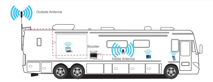
The Booster captures the signal from outside vehicle and boosts it to the phone. It takes the weak signal from your phone and boosts it back to the tower osting Your Cell Signal
